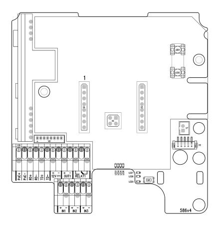
2N Access Unit Connectors, PCB Version 586v4
