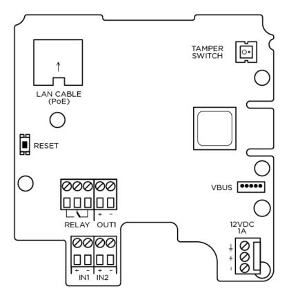
2N Access Unit Connectors, PCB Version 599v3
