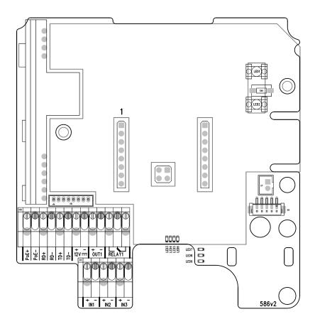
2N Access Unit Connectors, PCB Version 586v2
